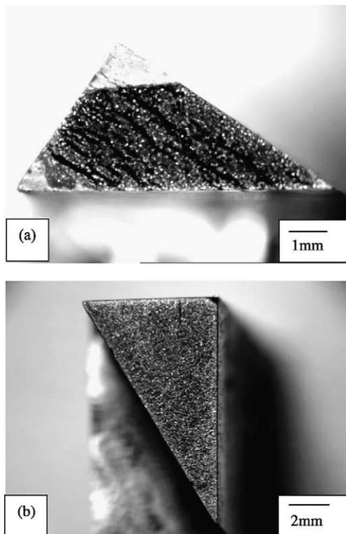
Fig. 4. The electrode surfaces after EDM: (a) copper–tungsten and (b) copper.
