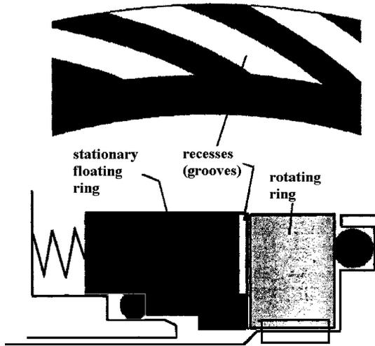
Fig. 1. Basic components of a film-riding gas seal [1].
