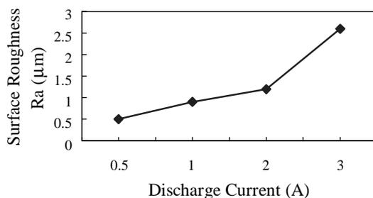
Fig. 8. Effects of discharge current on surface roughness when EDM WC.
