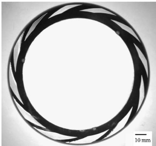
Fig. 12. Photograph gas seal ring face after EDM.
