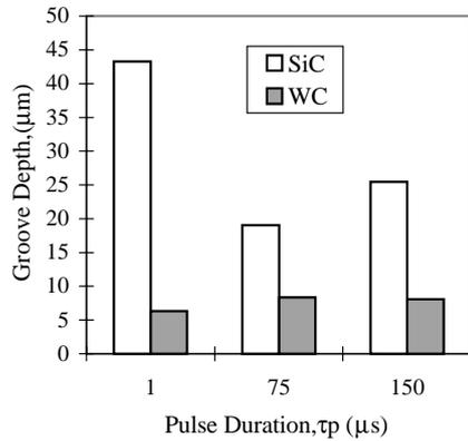
Fig. 7. Effects of pulse duration on groove depth for WC and SiC.
