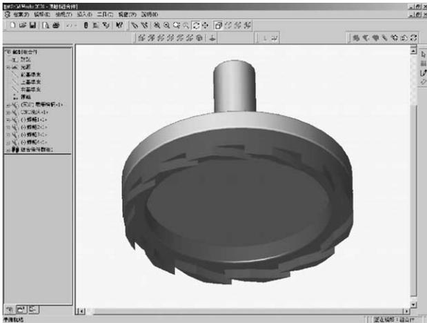
Fig. 11. CAD model of EDM electrode for gas seal ring face.
