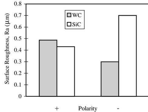
Fig. 5. Effects on surface roughness by electrode polarity with two different materials (WC and SiC).
