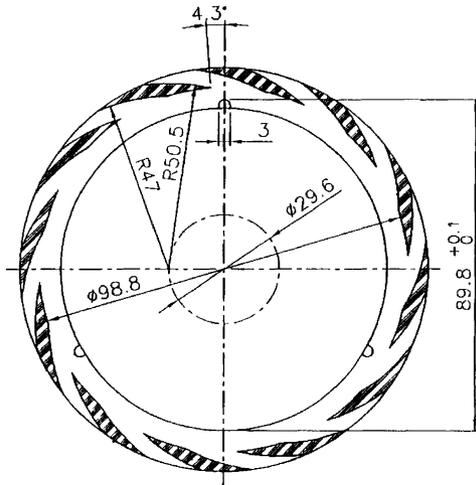
Fig. 10. Drawing of gas seal ring face.
