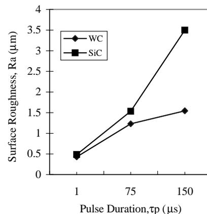
Fig. 6. Effects of pulse duration on surface roughness for WC and SiC.
