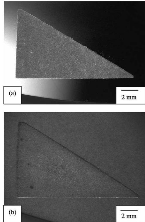
Fig. 9. The best workpiece surfaces after EDM: (a) WC and (b) SiC.
