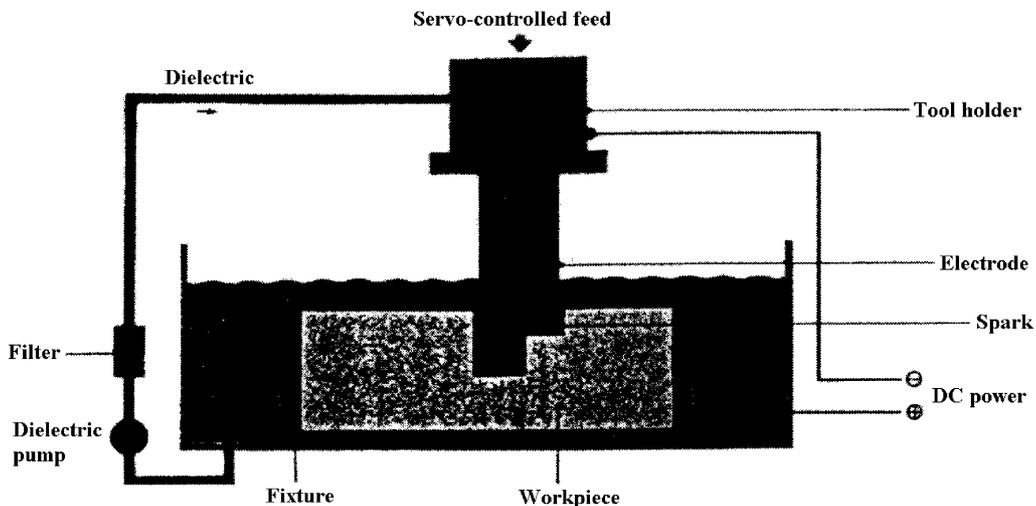
Fig. 3. Schematic diagram of the EDM process.
